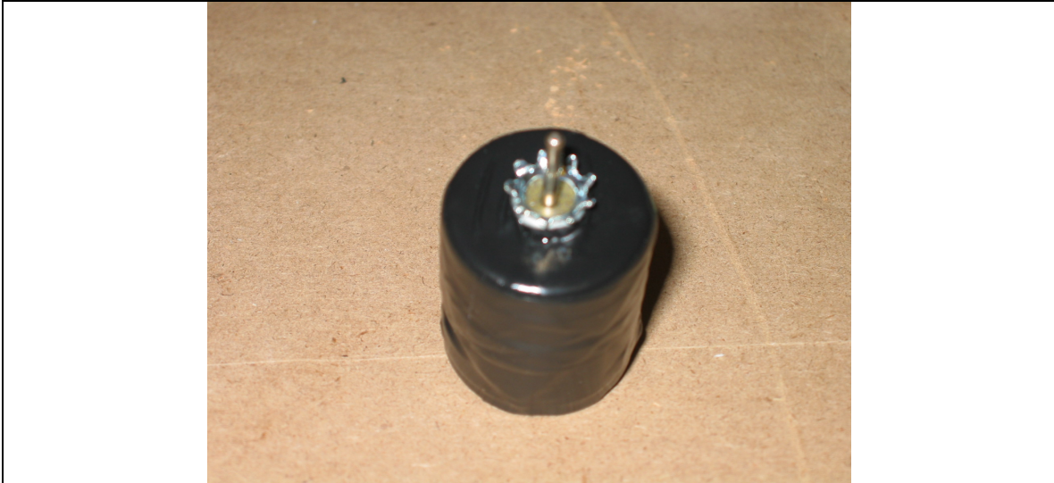
Figure 2 Spiked washer glued to motor
