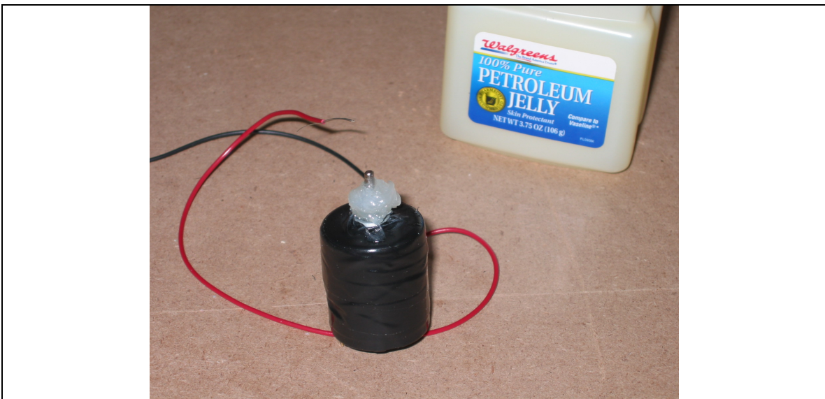
Figure 3 Petroleum jelly on shaft
